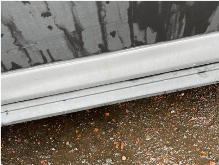
3: Sill os Dented Over 30mm
