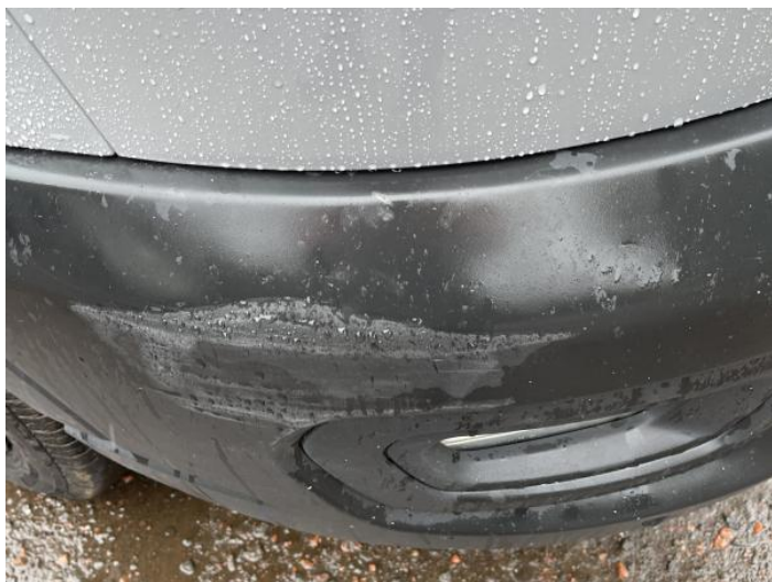
1: Bumper Front Moulding Scuffed (Unpainted) Over 100mm
